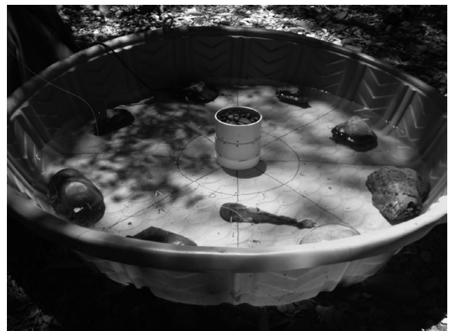
FIGURE 1 Experimental arena showing the acclimation chamber (center) and model sculpin (foreground)
